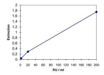
If the extinction of a serum sample lies above the value of calibrator 1 (200 RU/ml). The result shold be given as ">200 RU/ml". It is recommended that the sample be re-tested at a dilution of 1:400. The result in RU/ml read from the calibration curve for this sample must then be multiplied by a factor of 4.
